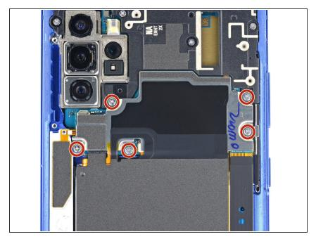
Use a Phillips screwdriver to remove the five 4 mm screws securing the wireless charging coil.
