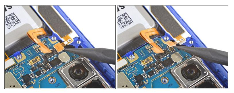
Use the pointed end of a spudger to disconnect the S-Pen charging coil connector from the motherboard.
