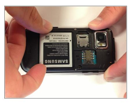
Place your finger on either bottom corner of the battery slot and lift to remove the battery.
