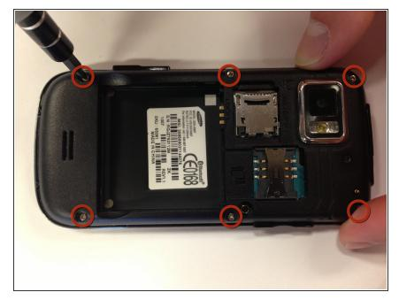
Using a Phillips #00 Screwdriver, remove the six 5 mm screws from the back casing of the phone.
