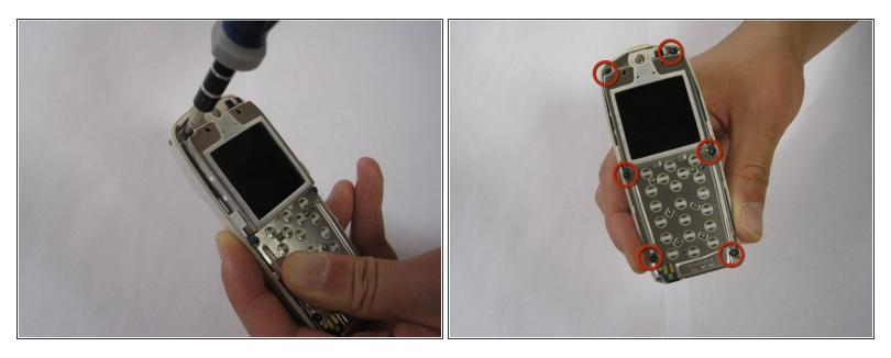
• Once the keypad has been removed, unscrew the 6 exposed screws on the front of the phone.
