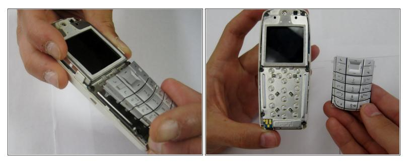
• Once the cover plate has been removed, the existing keypad should be easily removed.
