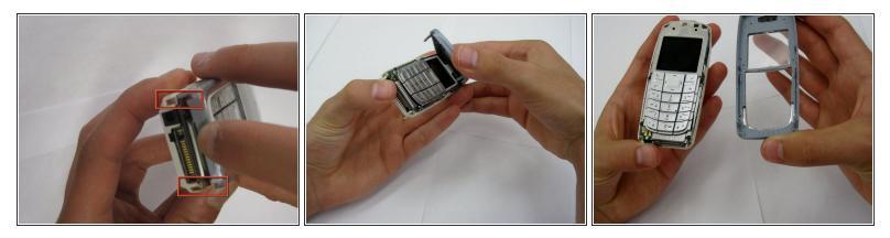
• Using your fingernails or another tool, pry the front face plate out along its edges and corners.
