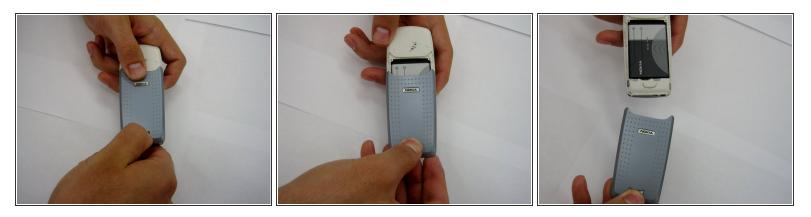
Remove the back cover plate of the phone. To do this press down the lock as you slide the cover toward the bottom of the phone.
