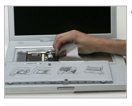
Pull the keyboard cable up from the logic board, holding the cable as close to the connector as possible.
