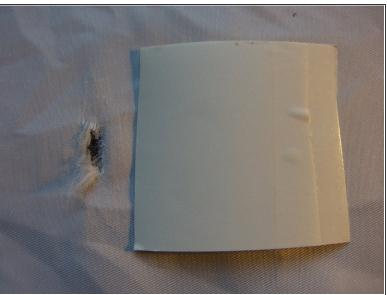
Cut a piece of sail tape to the length of the tear plus one inch excess.
