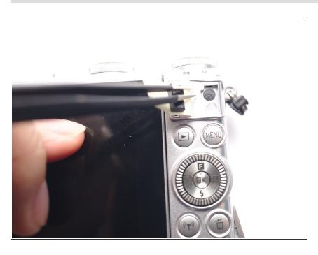
Peel here and remove 1 screw within.
