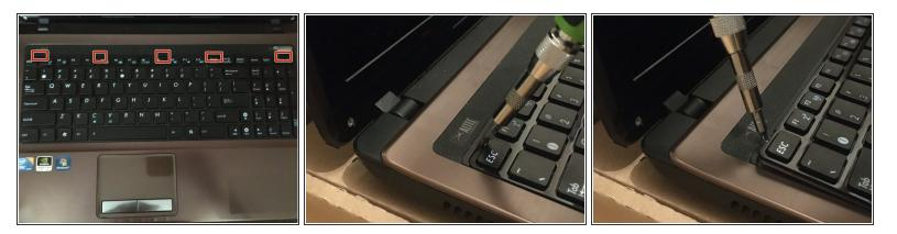
There are several pins holding the keyboard. Insert the tool at an angle, then turn it in the opposite direction to unclip them
