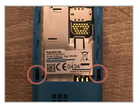
Push in the pins holding in the keypad
