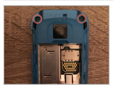
Remove the two T6 screws near the camera
