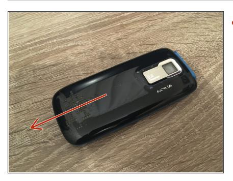
Slide the rear panel in the indicated direction to unlock it.
