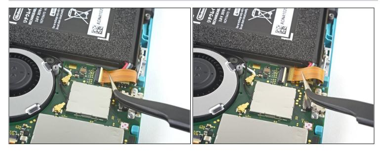
⚠ **Do Not Use Metal Tweezers!** Some fixers state that metallic tweezers can short circuit the ribbon cable/connector. It might be safer to just use nylon-tipped or ceramic-tipped tweezers.
