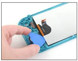
• Continue sliding the opening pick around the right edge of the LCD, slicing the adhesive.
