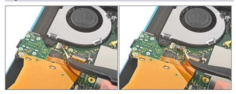
• Use a pair of tweezers to slide out the fan cable from its connector on the motherboard.
