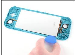
• Slide the opening pick along the top edge of the LCD to slice the adhesive.
