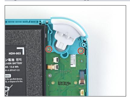
Use a JIS 000 driver or an official iFixit PH 000 driver to remove the two 4.5 mm screws securing the left trigger button assembly.
