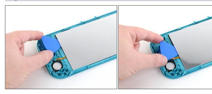
• Continue sliding the opening pick along the left edge of the LCD to slice the adhesive.
