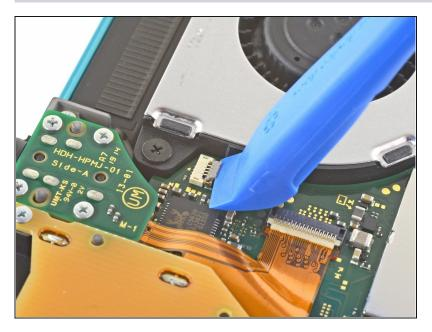
Use an opening tool or your fingernail to flip up the small, hinged locking flap on the fan cable's ZIF connector.
