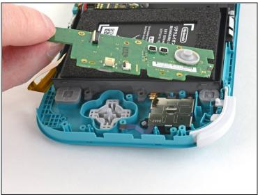
• Use your fingers to lift the daughterboard up and out of its recess to remove it.
