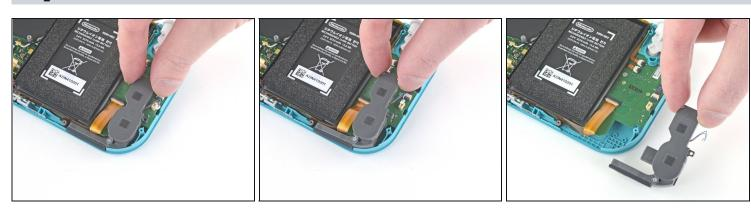
• Use your fingers to lift the speaker module up and out of its recess to remove it.
