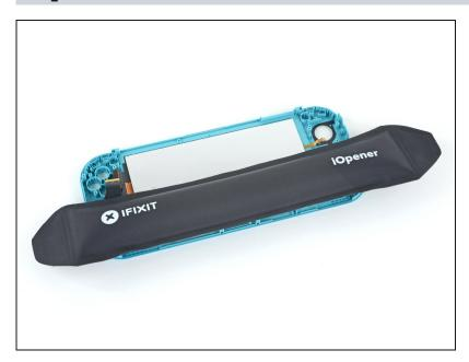
Apply a heated iOpener to the back side of the LCD along the bottom edge for 2 minutes.
