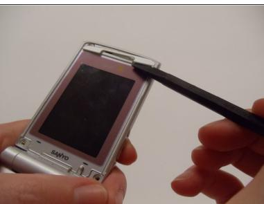
With the flat end of a spudger, remove the plastic covers located on the corners of the display near the hinge and above the screen, revealing four screws underneath.
