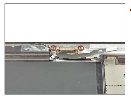
Remove the two 2.0 mm Phillips screws securing the dock connector to the rear case.
