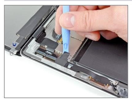
• Use a plastic opening tool to help remove the piece of tape covering the end of the dock connector cable.
