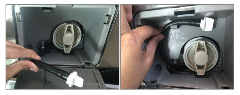
• Once the water stops coming out from the drain hose, secure it back into position.
