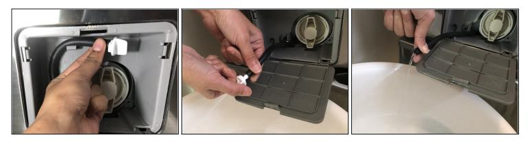
• Pull out the drain hose and unplug the white cap to let the excess water flow out into the basin.
