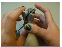
• Pull apart the inner hardware from the back case by prying on the left side.
