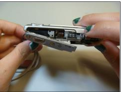
• Slide open the top panel. This is located on the top of the camera, where the power button and shutter button are.
