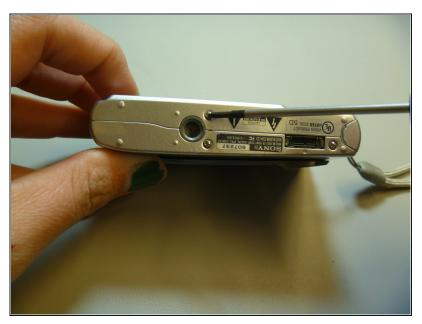
• Use screwdriver to remove screws.
