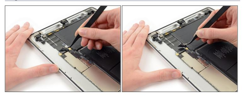
• If present, use <u>tweezers</u> to remove the piece of tape covering the end of the headphone jack/control board cable.
