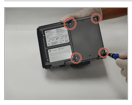
Remove the four 10mm screws from the bottom of the device with a Torx T10 screwdriver.
