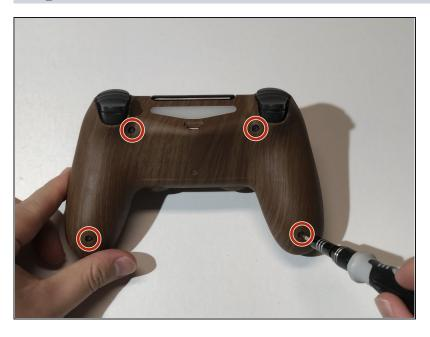
Remove the four 6 mm Phillips #00 screws on the back of the controller.
