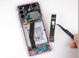
Gently peel up and remove the main and auxiliary flex cables.
