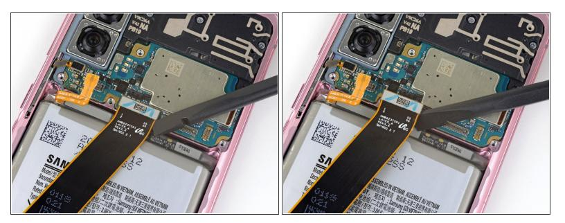
Use a spudger to pry up and disconnect the main display flex cable from the motherboard.
