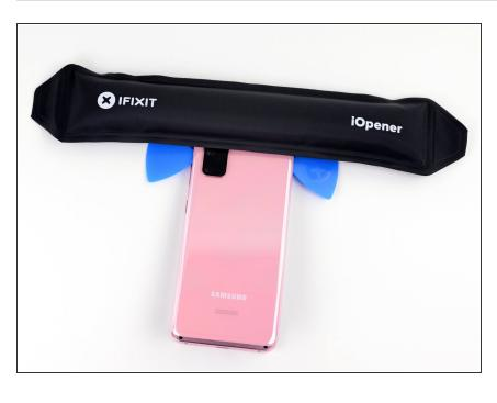
Apply a heated iOpener to the top edge of the back cover for two minutes.
