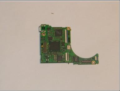
The motherboard can now be lifted out and separated from the rest of the camera.
