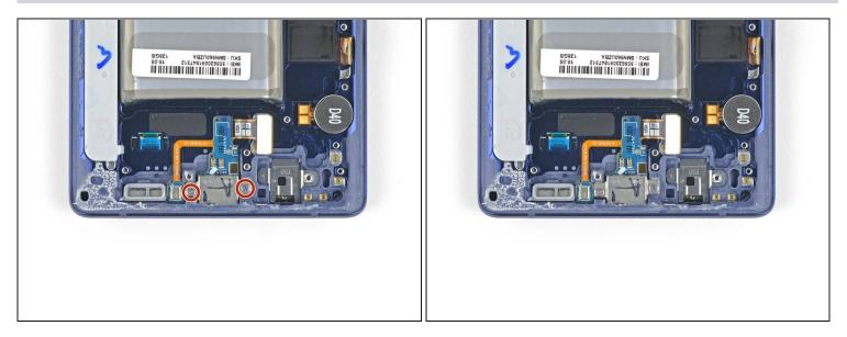
• Remove the two 3.2 mm Phillips screws from the charging assembly.
