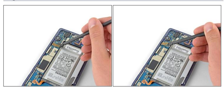
• Use the flat end of a spudger to disconnect the touchscreen cable from the motherboard.
