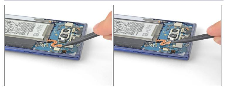
• Use the tip of a spudger to disconnect the orange ribbon cable connecting the battery to the motherboard.
