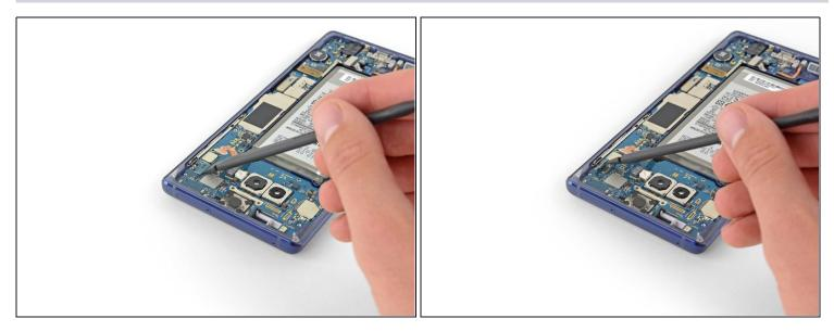
• Use the flat end of a spudger to pry the front sensor connector out of its socket.
