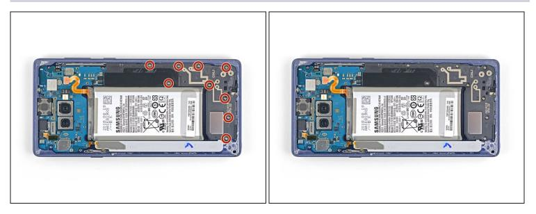
• Remove the nine 4 mm Phillips screws from the plastic cover next to the battery.
