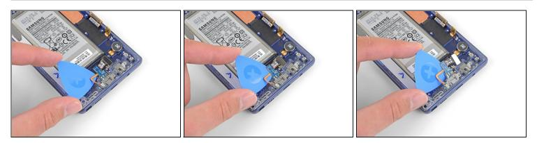
• Use an opening pick to separate the charging assembly from the phone.
