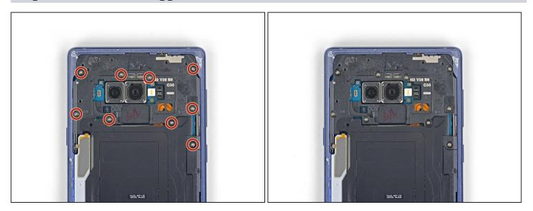
• Use a Phillips screwdriver to remove the nine 4 mm screws securing the upper midframe.
