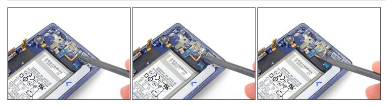
• Use a spudger to lift the microphone out from its housing.
