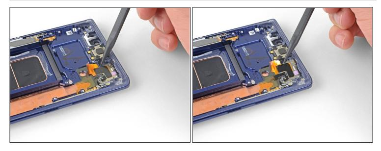
• Use a spudger to lift the left side of the front sensor array and separate the adhesive the rest of the way.
