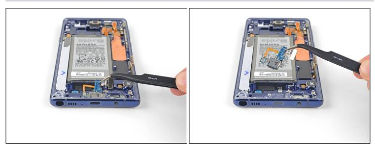
• Use a pair of <u>tweezers</u> to remove the charging assembly.
