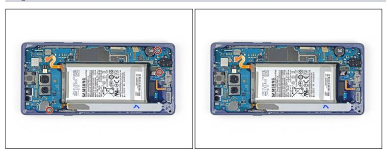
• Remove the three 4 mm Phillips screws securing the motherboard.
