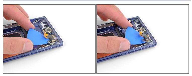
• Carefully slide an opening pick under the front sensor array ribbon cable to cut the adhesive underneath.
