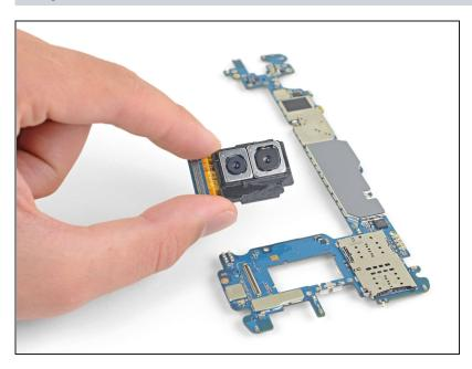
Remove the rear camera from the motherboard.
