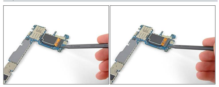
Use the tip of a spudger to pry the rear camera connector straight up and out from the motherboard.
