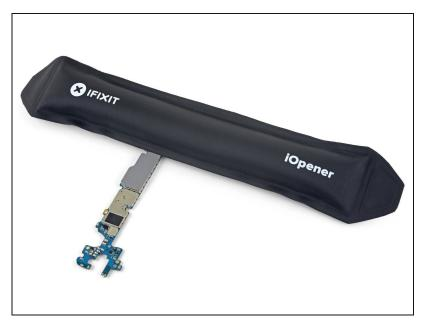
Use a heat gun or hair dryer or apply a heated iOpener for about a minute to soften the adhesive around the rear camera.
