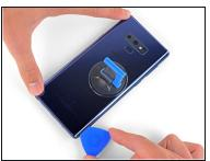
• Starting from the center, cut the adhesive up and down the right side with an opening pick.
