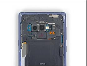
• Use a Phillips screwdriver to remove the nine 4 mm screws securing the upper midframe.
