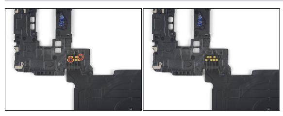
When assembling the new wireless charging coil, start by lining the posts on the midframe up with the holes in the coil to properly align the contacts on both components.
