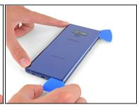
⚠ Be careful near the corner, as the glass is very weak. Apply more heat at any time if the adhesive becomes stuck.
