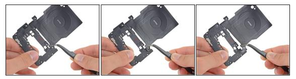
• Use a pair of tweezers to peel the upper-left corner of the wireless charging coil off the upper midframe.
