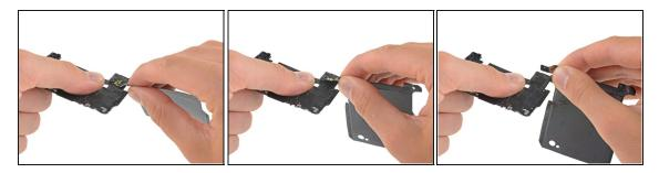
Peel the wireless charging coil off of the back of the upper midframe.
