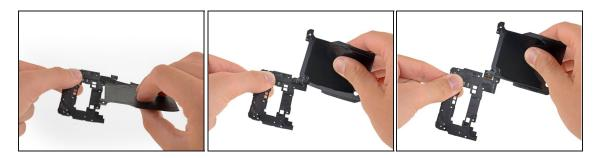
• Peel the wireless charging coil around the edge of the upper midframe.
