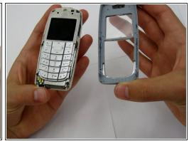
• Using your fingernails or another tool, pry the front face plate out along its edges and corners.
