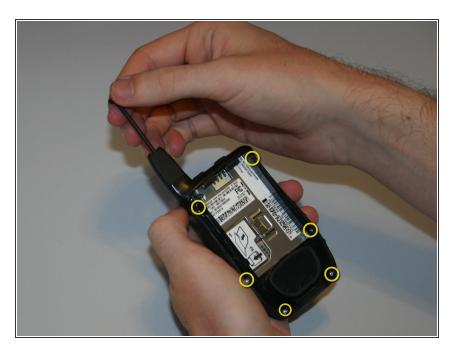
Pull antenna up, away from the phone, to reveal two of six screws.
