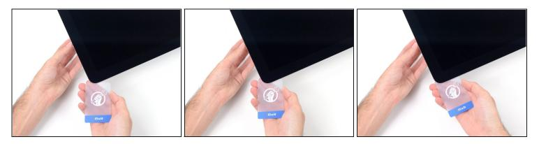
(i) While the opening tool cut most of the adhesive, the display will still be slightly adhered to the case. A <u>plastic card</u> will be necessary to free up the last of this adhesive.
