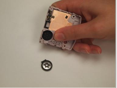
Gently tap the lower back casing on a hard surface to remove the speaker.
