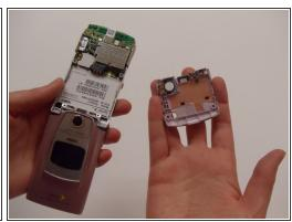
Remove the lower back cover to reveal part of the motherboard and the circular speaker housed in the back cover plate.
