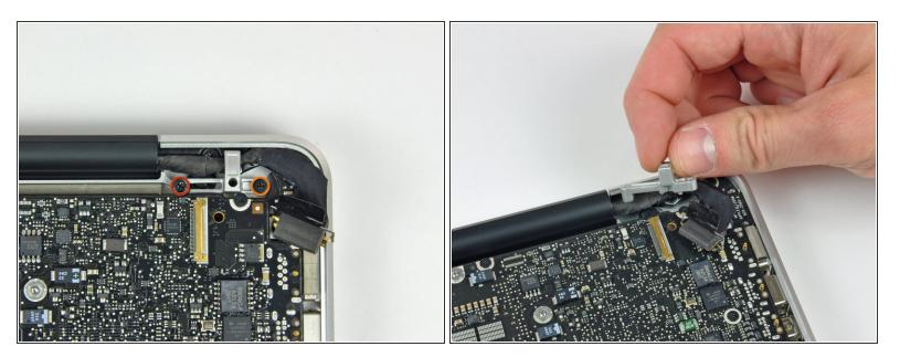
• Remove the following two screws securing the display data cable bracket to the upper case:
