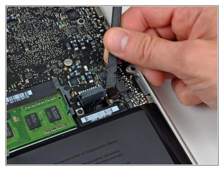
• Use the flat end of a spudger to pry the battery indicator cable connector up off the logic board.
