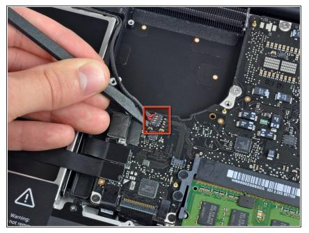
• Use the flat end of a spudger to pry the subwoofer and right speaker connector up off the logic board.
