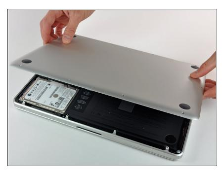
• Slightly lift the lower case and push it toward the rear of the computer to free the mounting tabs.
