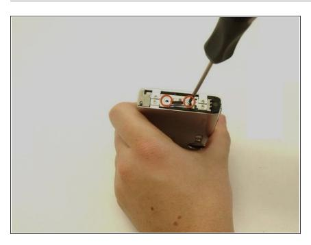
On the right hand side of the camera, remove the two screws from the wrist strap handle by using the Phillips screwdriver.
