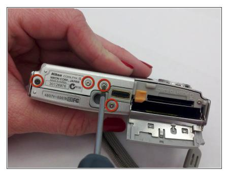
Use the Phillips screwdriver to remove the four screws on the bottom of the camera.
