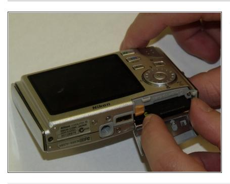
Press down on the SD card. This will cause it to eject, thus enabling it to be removed.
