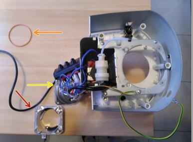
Once you removed the heating element you can replace the necessary pieces: bottom piece(red arrow), O-ring (orange arrow), upper piece (yellow arrow)
