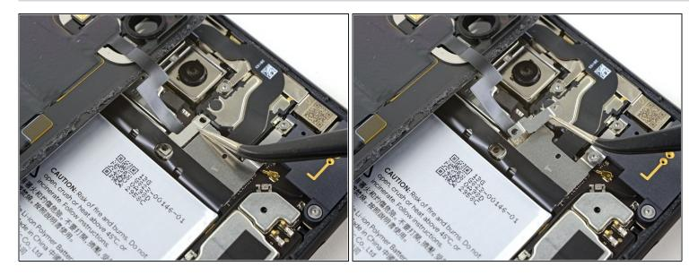
• Use a pair of tweezers to remove the back panel connector cover.
