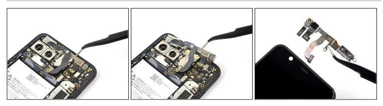
• Use a pair of tweezers to remove the front camera and sensor assembly.
