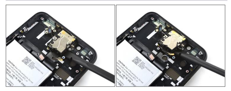
• Using the flat end of a spudger, pry the earpiece module away from the phone's midframe.
