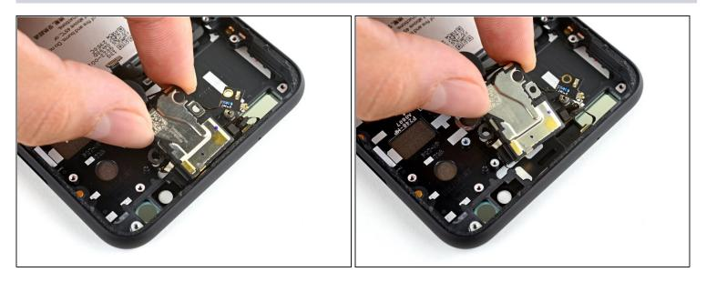
Pull the earpiece speaker away from the light adhesive holding it to the phone's top frame.
