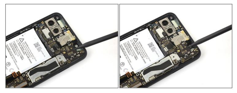
• Using a spudger, pivot the top end of the motherboard up and out of the phone's frame.
