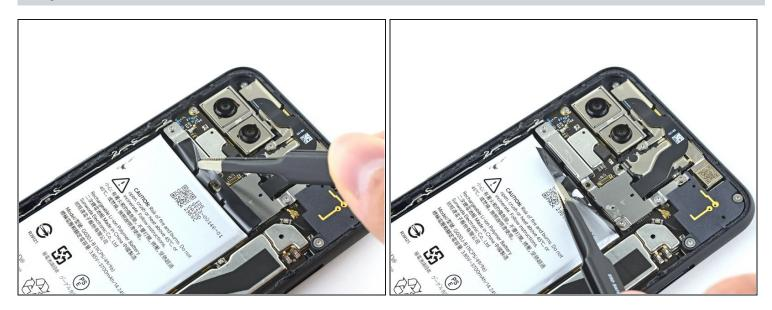
Gently pry back the battery adhesive pull tab to allow easier access to the screws underneath it.
