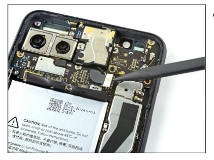
• Disconnect the earpiece speaker connector from the motherboard.
