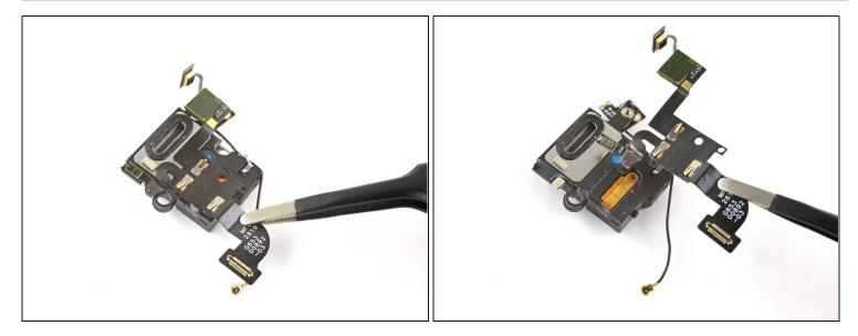
• Use a pair of tweezers to peel away and remove the Soli motion sensor cable, which is held in place with some light adhesive, leaving just the earpiece speaker.
