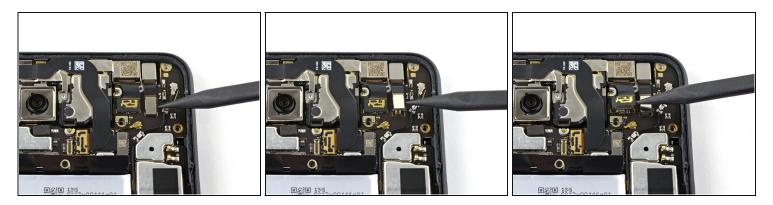
• Using the pointed end of a spudger, pry the camera and sensor connectors straight up from the motherboard.
