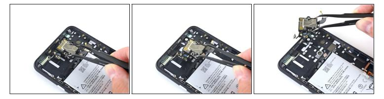
• Use a pair of tweezers to remove the earpiece speaker and Soli motion sensor assembly.
