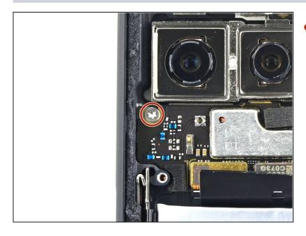
• Use a T3 Torx driver to remove the 2.7 mm screw securing the motherboard to the frame.
