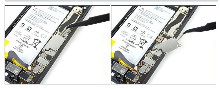
• Use a pair of tweezers to remove the display connector cover.
