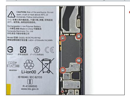
Use a T3 Torx driver to remove the four 3.5 mm screws securing the display connector cover.
