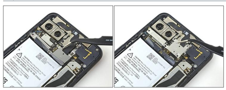
• Use a pair of tweezers to remove the rear-facing camera connector cover.
