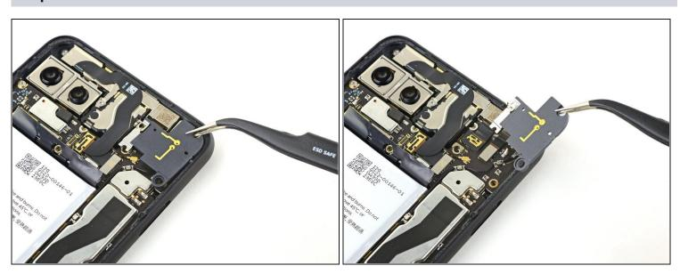
• Use a pair of tweezers to remove the front-facing camera connector cover.
