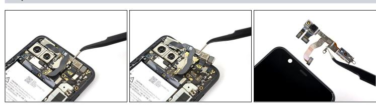
Use a pair of tweezers to remove the front camera and sensor assembly.
