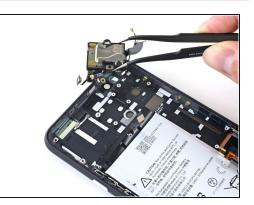
Use a pair of tweezers to remove the earpiece speaker and Soli motion sensor assembly.
