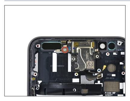
Use a T3 Torx driver to remove the 2 mm screw securing the small earpiece module board to the phone.
