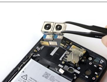
Use a pair of tweezers to remove the rear-facing camera module.
