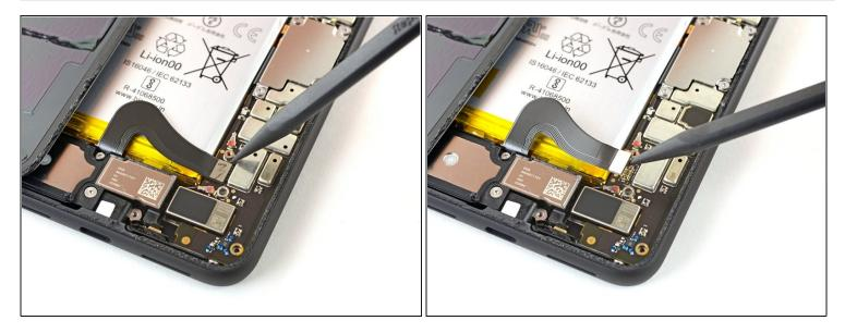
⚠ Whenever you use the spudger near the battery, be very careful not to puncture the battery.
