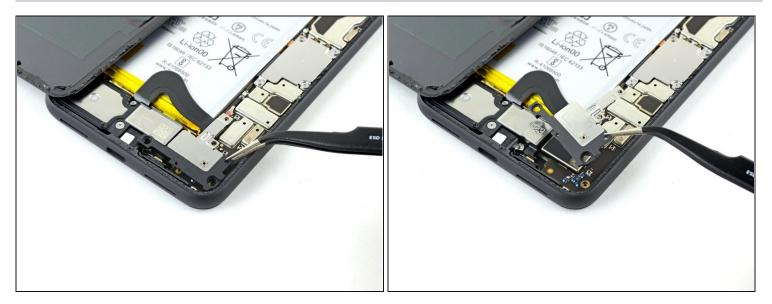
• Use a pair of <u>tweezers</u> to remove the battery connector shield.
