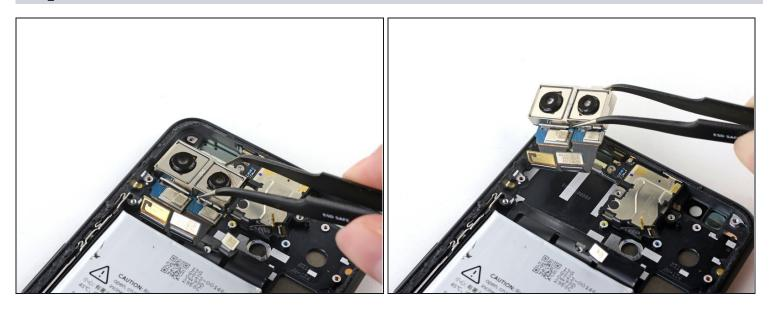
• Use a pair of <u>tweezers</u> to remove the rear-facing camera module.
