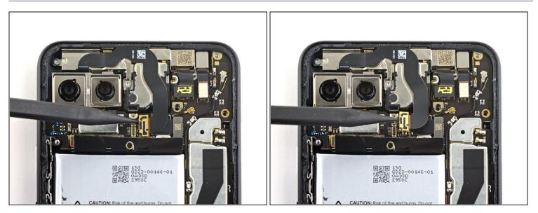
• Disconnect the additional sensor connector.
