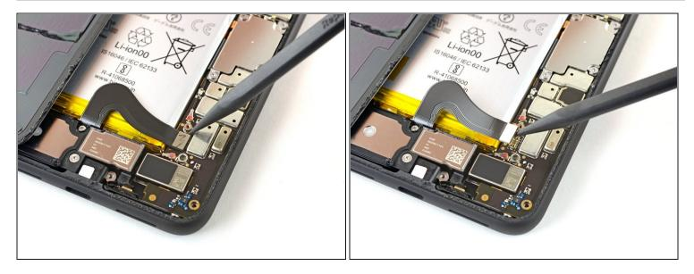
A Whenever you use the spudger near the battery, be very careful not to puncture the battery.
