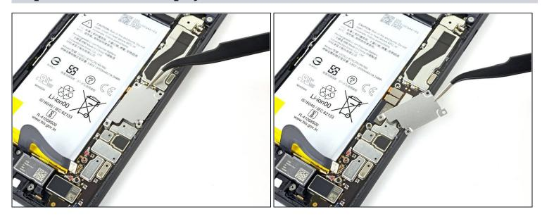
• Use a pair of <u>tweezers</u> to remove the display connector cover.
