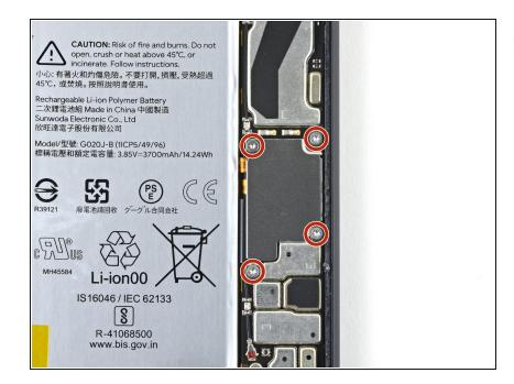
Use a T3 Torx driver to remove the four 3.5 mm screws securing the display connector cover.
