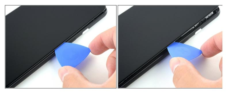
• Insert a third opening pick under the display assembly in the middle of the right edge of the phone and twist to separate the assembly.
