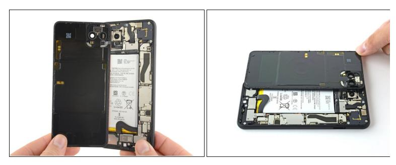
• Continue swinging open the back panel until you can rest it on the left edge the phone, being careful not to put any stress on the attached ribbon cable.
