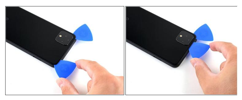
Slide the third opening pick around the top right corner and across the top side of the phone, slicing the final strip of adhesive.
