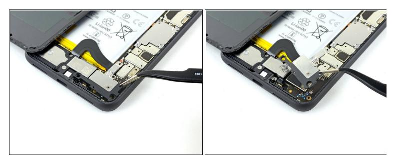
• Use a pair of tweezers to remove the battery connector shield.
