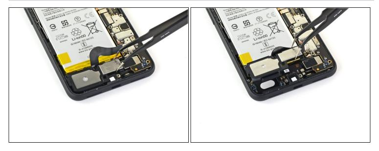
• Use a pair of tweezers to remove the loudspeaker.
