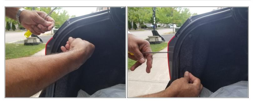
Push the carpet back in place and screw in the two fasteners to secure the trunk liner.
