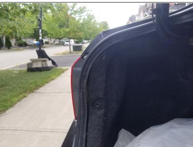
Open the trunk lid and remove the two black plastic fasteners on the side of the car with burnt out lights using a flat head screwdriver.
