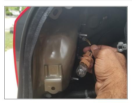
Replace the new bulb and push it in the socket.
