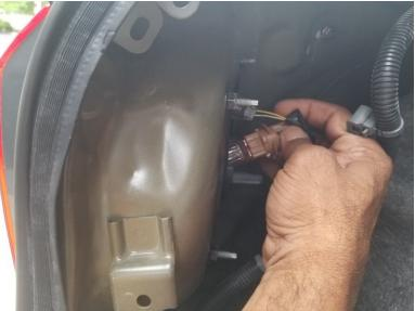
Turn the brake light counterclockwise and pull the old light straight out of the socket.
