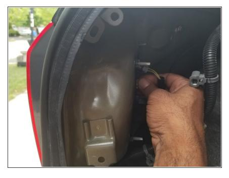
Turn the socket clockwise while placing it in the housing.
