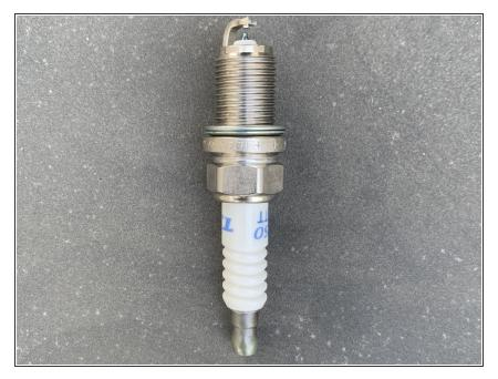
• Inspect the new spark plug to ensure that it is completely dry.
