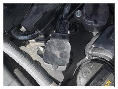
• Connect the wire back to the spark plug.
