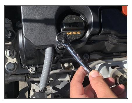
• Place the engine cover over the engine and reinstall the bolts using the wrench.
