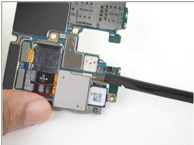
Pry up and disconnect the ultrawide camera connector from the motherboard.
