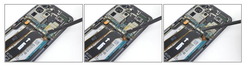
• Use a spudger to pry up and disconnect the main and auxiliary flex cables from the motherboard.
