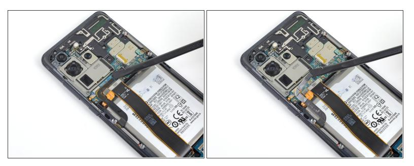
Pry up and disconnect the left 5G antenna cable from the motherboard.
