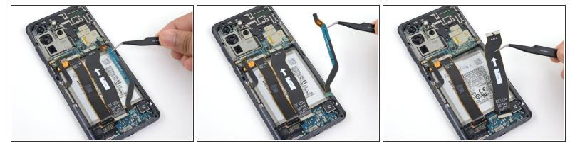
Gently peel up and remove the main and auxiliary flex cables.
