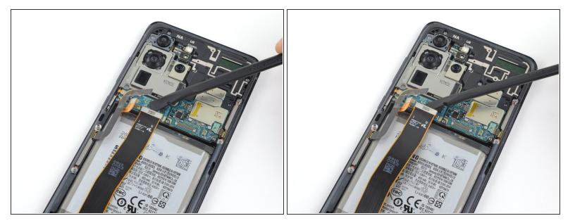
Pry up and disconnect the main display flex cable from the motherboard.
