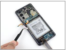
Gently peel up and bend the display and left 5G antenna flex cables out of the way of the motherboard and battery.
