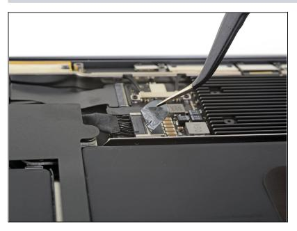
Peel back the tape covering the battery connector enough to reveal the connector underneath.
