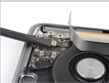
Use the flat end of a spudger to pry the Touch ID sensor connector straight up and disconnect
