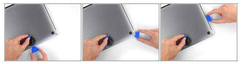
• Repeat the previous step on the other side, using an opening pick to to release the second clip.
