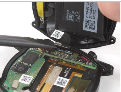
Use a spudger to pry up and disconnect the distribution cable connector.
