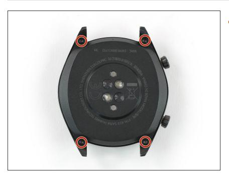
Remove the four Torx T3 screws (3.65 mm length).
