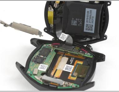
Use a pair of tweezers to remove the metal shield which covers the flex connector of the distribution cable.
