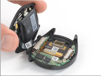
Carefully fold the back cover assembly to the side of the two watch crowns.
