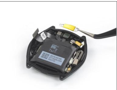
Use a pair of tweezers to remove the metal shield which secures the battery connector.
