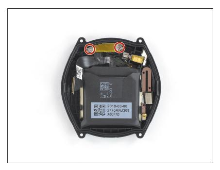
Remove the two Phillips #00 screws (2.6 mm length).
