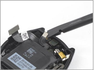
Use a spudger to pry up and disconnect the battery flex connector.
