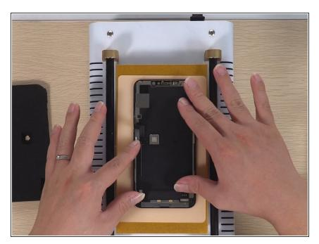
Heat up the screen on the heating platform. Here please be noted that the temperature of the heat platform should be at 90°C.
