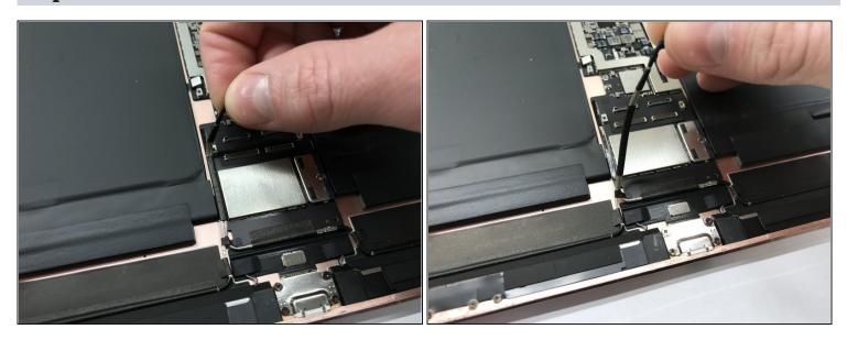
• Gently pull up on the antenna coax cable to separate it from the logic board.
