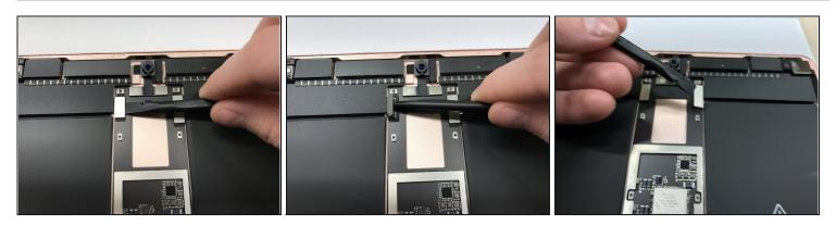
Disconnect the top left & right sensor array front panel connectors (FPC).
