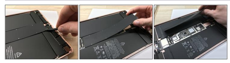
• Remove the logic board shield
