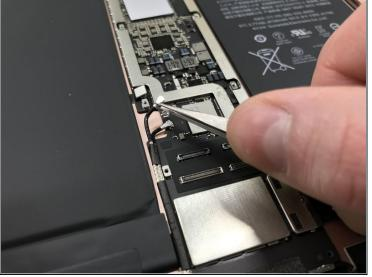
• Use <u>tweezers</u> to disconnect the antenna connectors.
