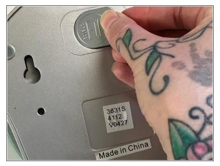
• Once the battery is secured, replace the battery cover.
