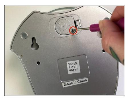
• Using the Phillips #00 screwdriver once again, replace the screw that secures the covering.
