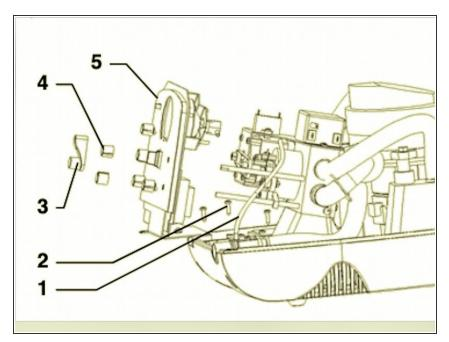
Unscrew the three 12.7mm plastite screws (2) holding the panel assembly to the lower housing. A long Phillips screwdriver is very helpful for access to the three screws. (Page 3)
