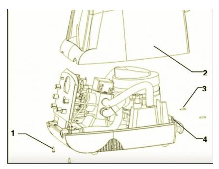
First, remove the two 16mm pan head screws (1) directly under the front panel of the ventilator. (Page 3).
