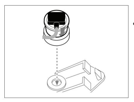
Ensure that the new rubber seal is intact, then firmly put in a new bacterial filter.
