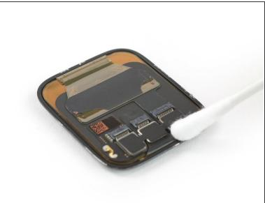
Apply a little bit of high isopropyl alcohol (>99%) to a Q-tip or use a <u>cleaning pad</u> to gently remove the adhesive leftovers from the Force Touch gasket on the case and on the screen.
