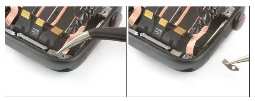
Use a pair of tweezers to remove the metal plate which covers the Force Touch gasket connector.
