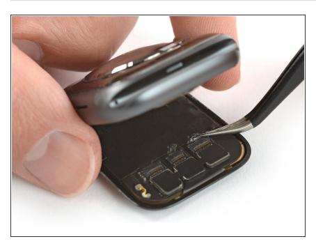
Use a pair of tweezers to carefully peel off the tape covering the three display cable connectors.
