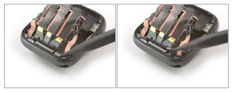
• Use the pointed end of a spudger to pry the Force Touch gasket connector out of its socket.
