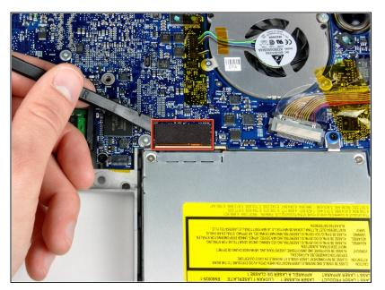
Use the flat end of a spudger to disconnect the orange SuperDrive ribbon cable from the logic board, removing tape as necessary.
