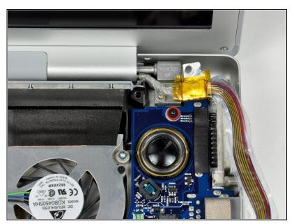
Remove the single black 6 mm T6 Torx screw securing the upper portion of the logic board to the lower case.
