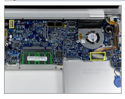
Disconnect the iSight and display data cables from the logic board by sliding them straight back out of their connectors, removing tape as necessary.
