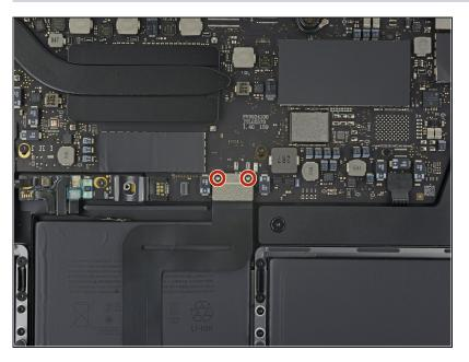
Use a T5 Torx driver to remove the two 1.9 mm screws securing the trackpad cable connector bracket.
