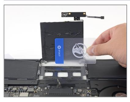
• Use the card to lift the battery cell until it fully separates from the aluminum case.
