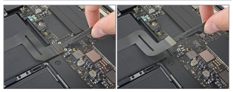
• Use a spudger to disconnect the trackpad ribbon cable by gently prying its connector straight up from the logic board.
