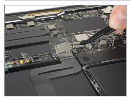
Remove the trackpad cable connector bracket.
